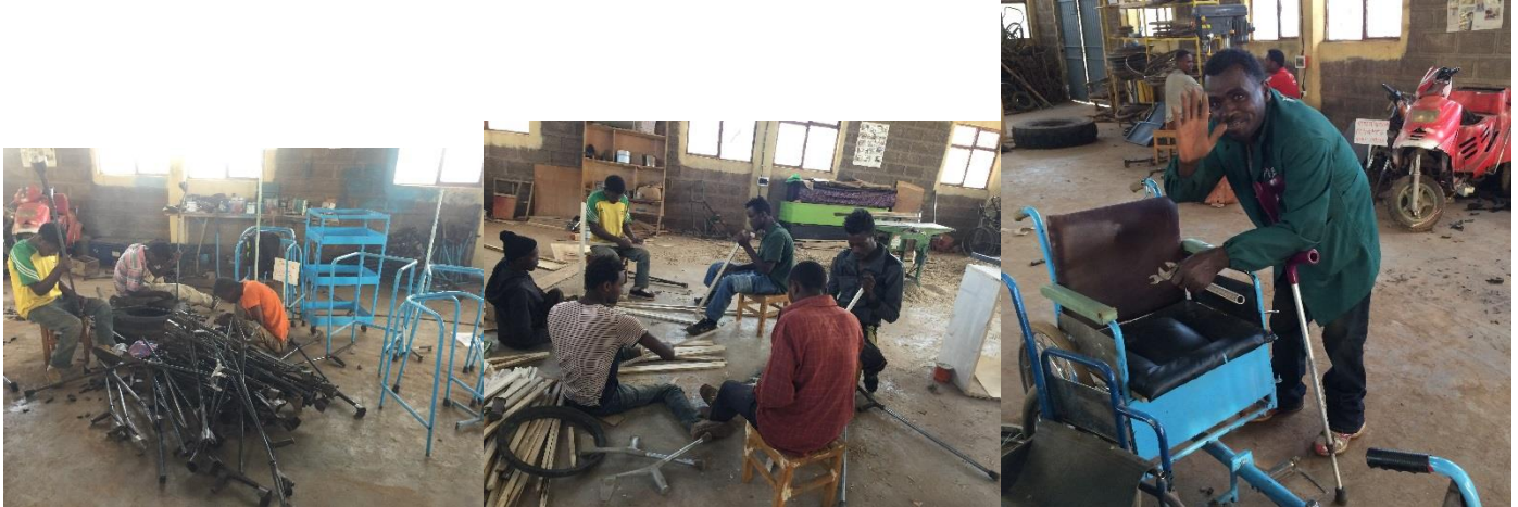
Manufacturing crutches in the workshop: Lower and upper arm walking sticks....
